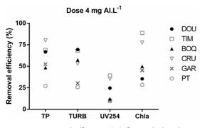
**Figure 2.** Removal efficiency (%) for total phosphorus (TP), turbidity (TURB), humic substances  $(UV_{254})$  and chlorophyll-a (Chl-a) in raw water from Dourados (DOU), Timbaúba (TIM), Boqueirão (BOQ), Cruzeta (CRU), Gargalheiras (GAR) and Passagem das Traíras (PT) reservoirs, after coagulation-flocculation with the dose of 4 mg Al L<sup>-1</sup> and 30 minutes of sedimentation.
