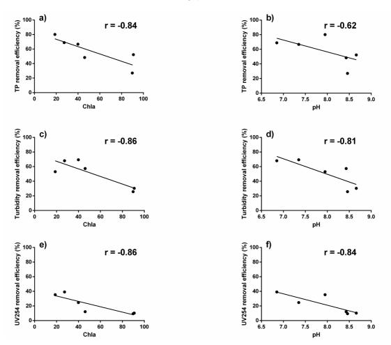
**Figure 3.** Correlations between chlorophyll-*a* concentration and pH with total phosphorus (TP), turbidity and  $UV_{254}$  removal efficiency (%) based on the dose of 4 mg Al L<sup>-1</sup>.
