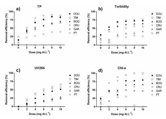
**Figure 1.** Removal efficiency (%) for total phosphorus (TP), turbidity, humic substances (UV<sub>254</sub>) and chlorophyll-a (Chl-a) in raw water from Dourados (DOU), Timbaúba (TIM), Boqueirão (BOQ), Cruzeta (CRU), Gargalheiras (GAR) and Passagem das Traíras (PT) reservoirs, after coagulation-flocculation with different concentrations of aluminium (0, 2, 4, 6, 8 and 10 mg Al L<sup>-1</sup>) and 30 minutes of sedimentation.
