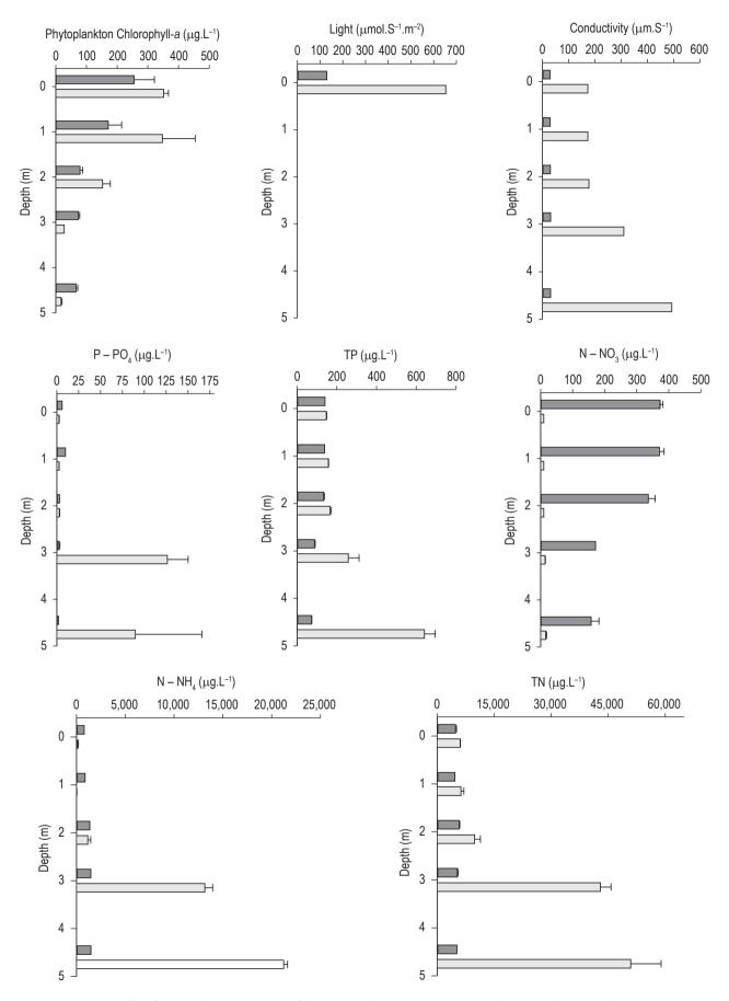
Figure 3. Vertical profile of mean values (n = 2, SD) of abiotic variables at Garças Reservoir during the dry () and rainy period ().
